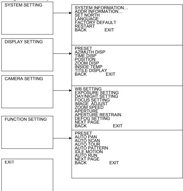
The above diagram illustrates the overall structure of the speed dome setup menu.
