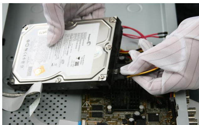
Figure 2-3 Connect Power Cable
