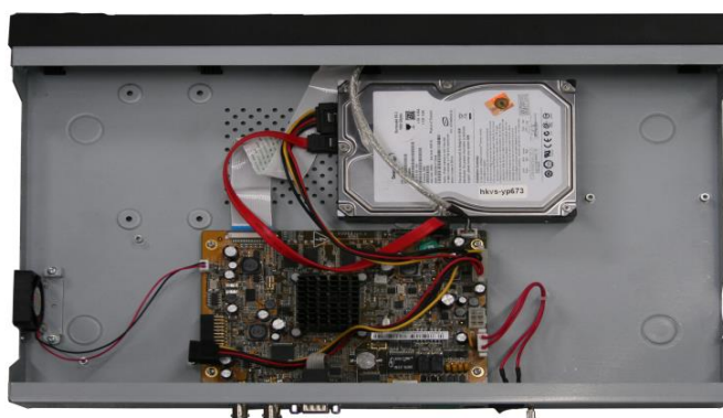
Figure 2-4 Fix Hard Disk
