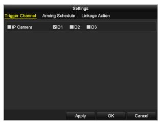
Figure 8-2 Set Trigger Camera of Motion Detection
