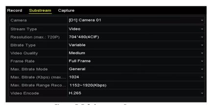
Figure 5-5 Sub-stream Parameters
