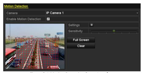
Figure 8-1 Motion Detection Setup Interface
