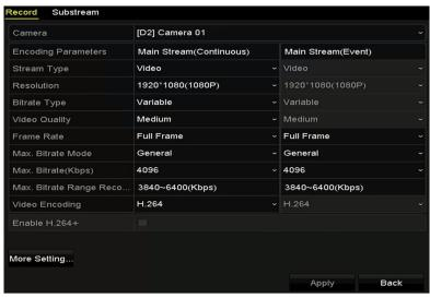
Figure 5-3 Recording Parameters
