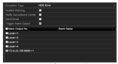
Figure 12-27 Configure HDD Error Alarm
