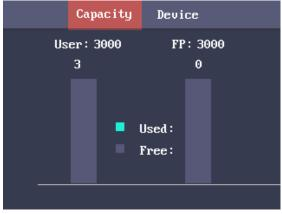
**User Capacity:** The maximum user amount that can be configured. *Note:* The default maximum user amount is 3,000. **Fingerprint Capacity:** The maximum fingerprint amount.
