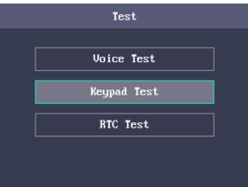
2. Press the OK button to start testing. If the keypad test succeeds, the screen will display the corresponding numbers or functions of the pressed key.
