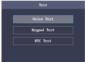
2. Press the OK key. If the device voice is working properly, you are able to hear "Voice Test Success".
