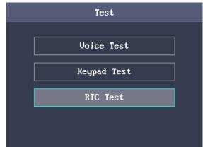
2. Press the OK key to enter the RTC Test interface. If the test succeeds, the screen will display the synchronization time.
