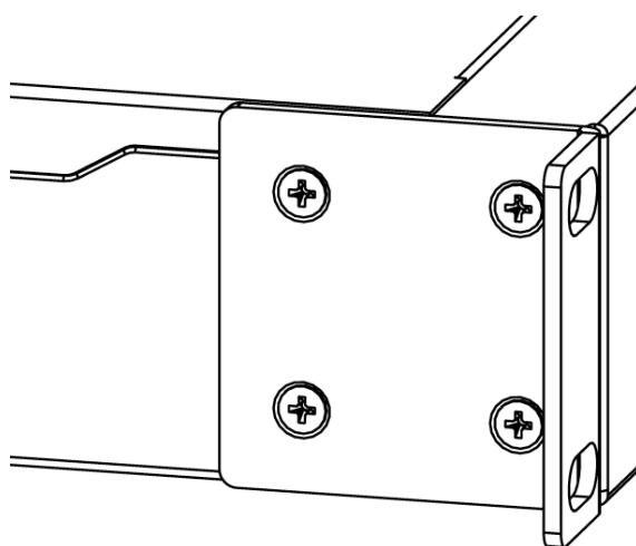
2. Place the device in rackmount enclosure and align with the holes so that device fits conveniently;
