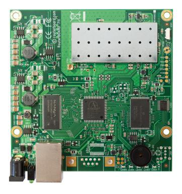
The RB711 is a small RouterBOARD wireless router with an integrated 5GHz 802.11a/n wireless card.
